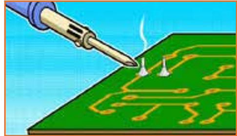
Fig 3.2.13: Assembly of Board and Components
