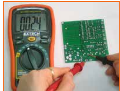
Fig 4.2.8: Measure Voltage & Resistance
