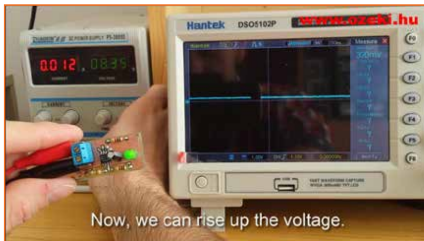
Fig 4.2.11: Checking PCB by oscilloscope
