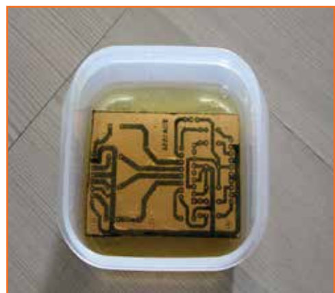
Fig 3.2.9: Perform Final Etching
