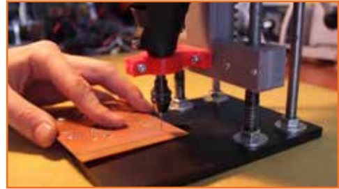
Fig 3.2.7: Drill Holes in Board
