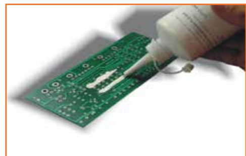
Fig 3.2.11: Apply the Solder Mask
